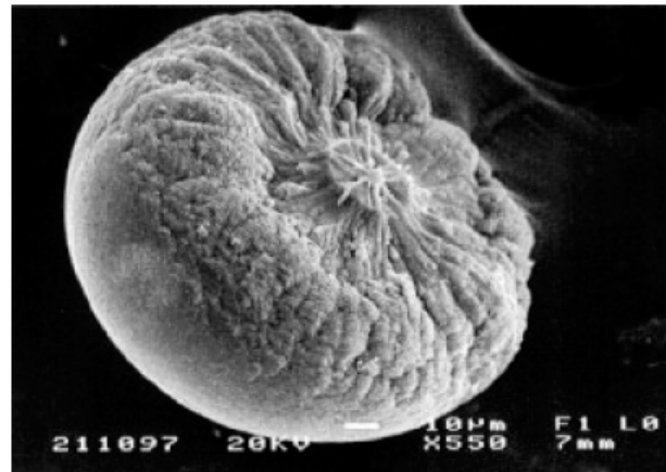
Fig. 4. SEM image showing half of an equatorially notched fluorapatite-gelatin spheroid. Scale bar is 10 µm. Reproduced with permission from Chemistry of Materials [30]. Copyright 2001 American Chemical Society.
